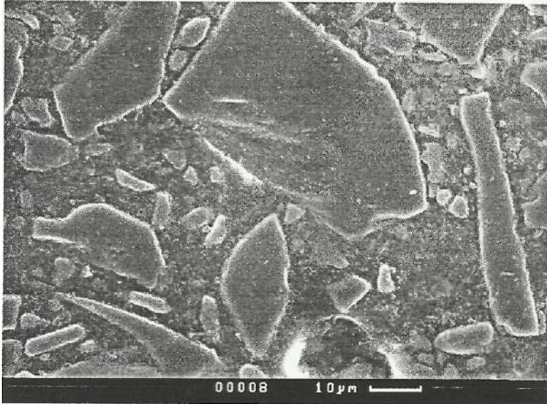
Figure 11: Scanning Electron Microscopy-Back Scatter Imaging of 100% GGBFS at 140°C for 28 Days X1000.
