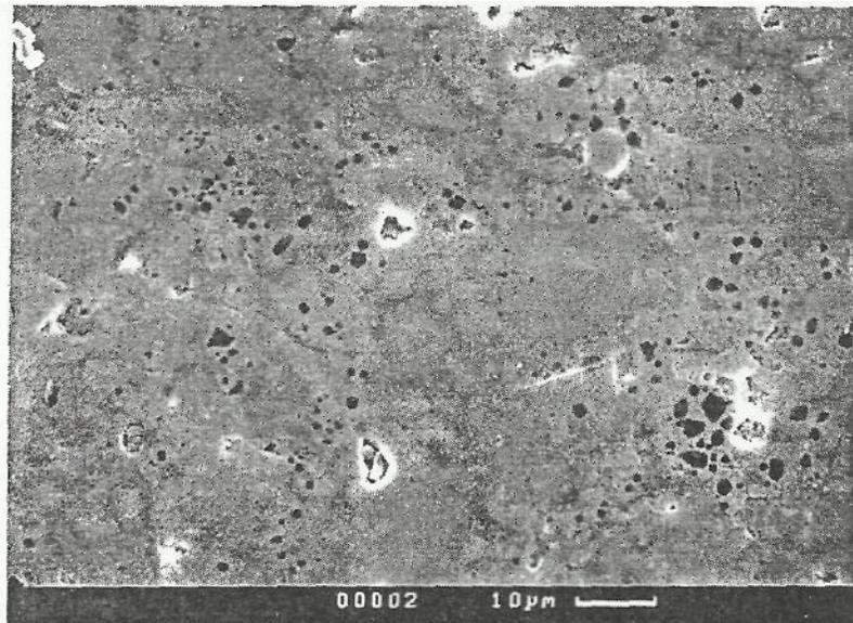
Figure 10: Scanning Electron Microscopy-Back Scatter Imaging of 100% OPC at 140°C for 28 Days X1000.
