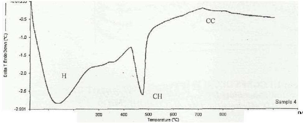
Figure 6: DTA Trace of 100% OPC at 80°C for 28 Days
