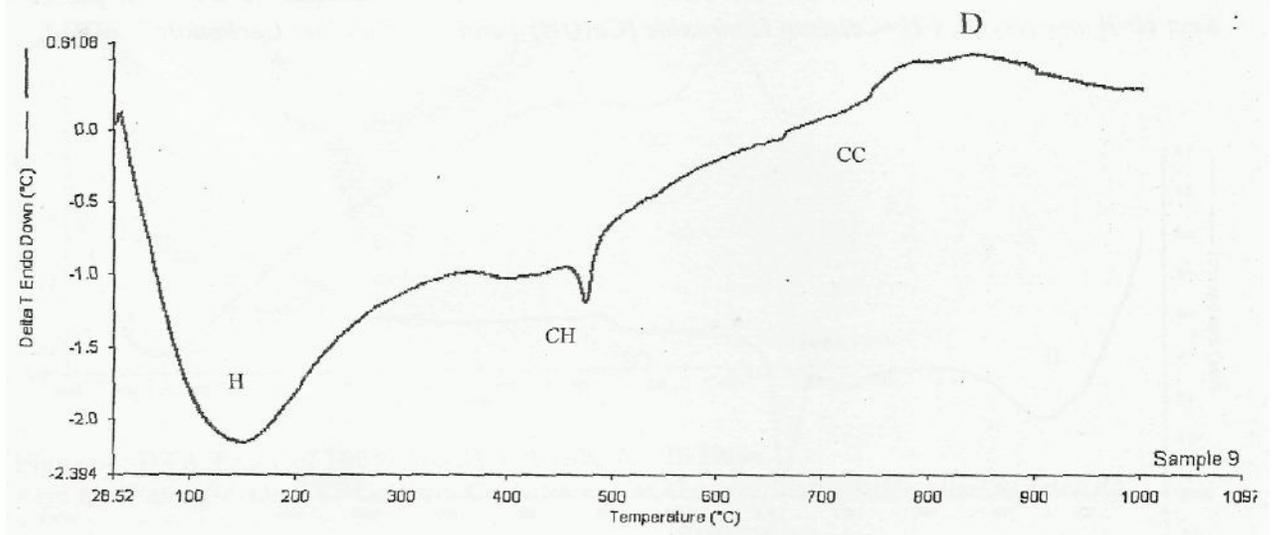
**Figure 9: DTA Trace of 1:1 GG15FS/OPC at 140°C for 28 Days**
