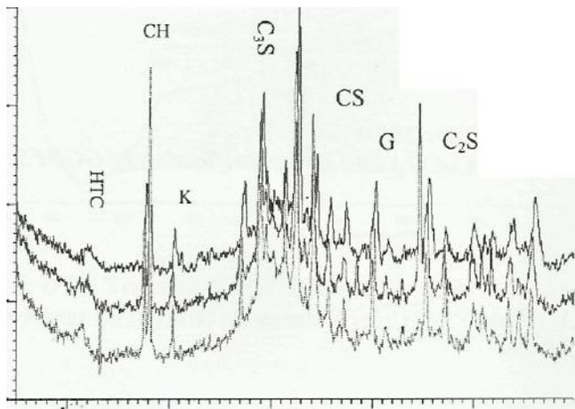
**Figure 3: XRD Trace of 1:1 GGBFS/OPC at 28 Days**
