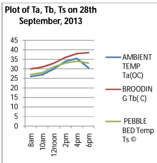
**Appendix (b) Graphs of Ambient temp, Ta, Brooder temp Tb and pebble bed temp Ts on different times of the day on 28<sup>th</sup> Sept. 2013**
