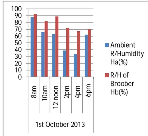
**Appendix (e) Plot of relative humidity of the Ambient Ha and relative humidity of the brooder on 1<sup>st</sup> Oct 2013 at different times of the day.**
