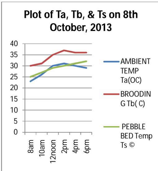
**Appendix (d) Graphs of Ambient temp, Ta, Brooder temp Tb and pebble bed temp Ts on 8<sup>th</sup> Oct. 2013 at different times of the day.**
